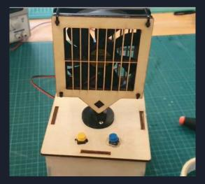
Laser cut- box housing, fan grill 3D Print- Fan stem, stem mount
